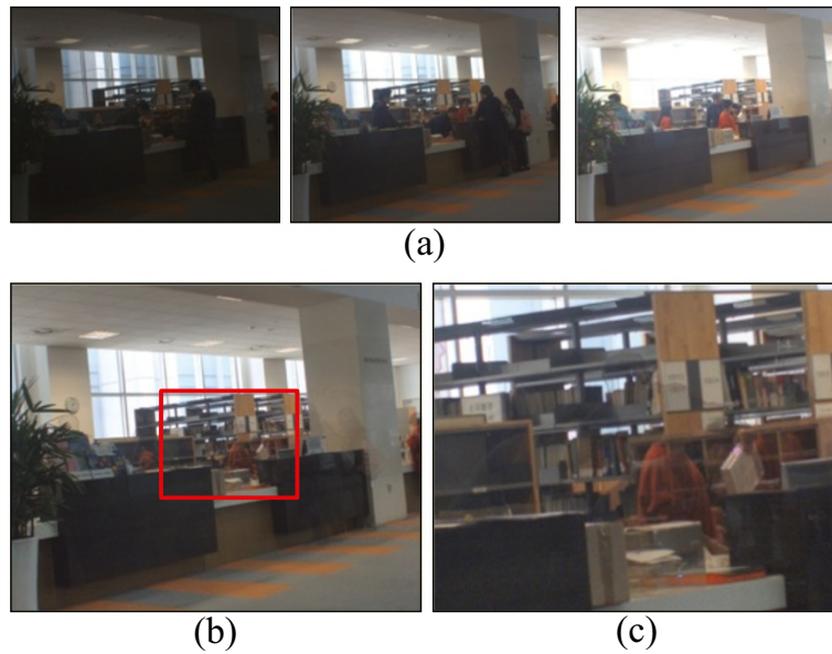
Figure 7 An example of the ghost artifact in an HDR image. (a) Input images, (b) the result containing ghost artifact, and (c) close-up of the red box in (b) .
