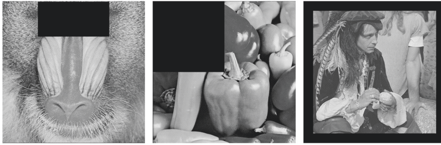
Fig. 13 Robustness of the DWT-DCT technique against different types of cropping. The BCR values is 100 % for these attacks
