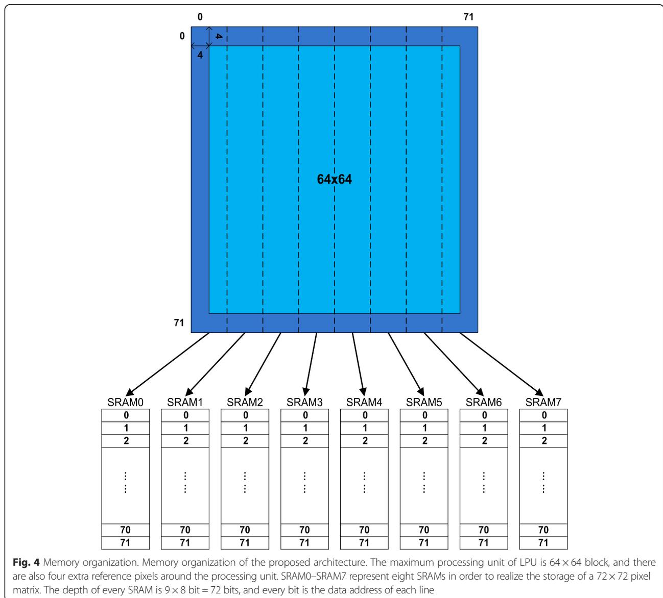
depth of every SRAM is  $9 \times 8 \text{ bit} = 72 \text{ bits}$ , and every bit is the data address of each line. There are eight SRAMs in order to realize the storage of a  $72 \times 72$  pixel matrix. Based on this organization, only SRAM0 and SRAM1 are open for  $8 \times$  processing unit while the others are close with no data access. Only when the width of processing unit is 64, all the SRAMs will be used to store and read the input reference pixels.
