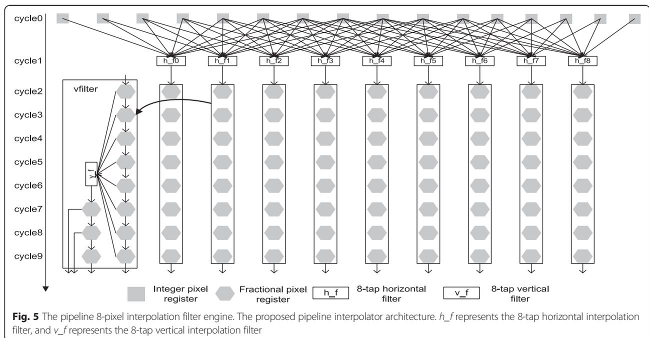
execute the filtering operation on the reference pixels from line 2 to line 9.
