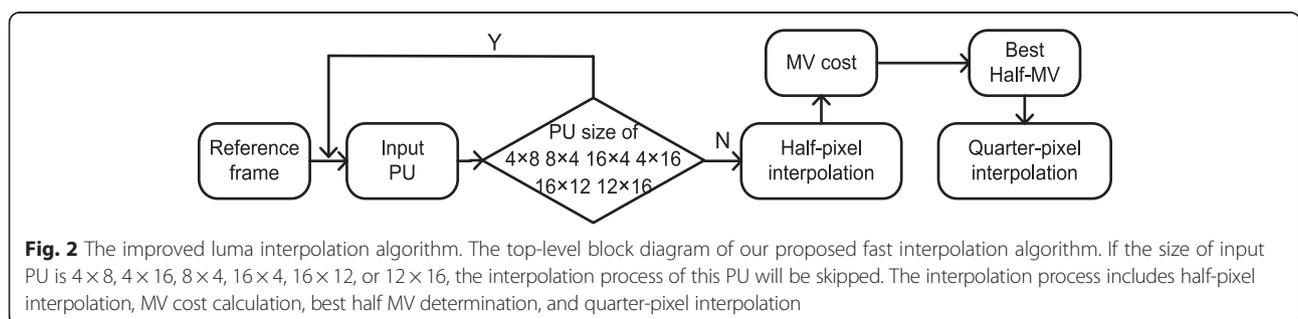
**Fig. 2** The improved luma interpolation algorithm. The top-level block diagram of our proposed fast interpolation algorithm. If the size of input PU is 4 × 8, 4 × 16, 8 × 4, 16 × 4, 16 × 12, or 12 × 16, the interpolation process of this PU will be skipped. The interpolation process includes half-pixel interpolation, MV cost calculation, best half MV determination, and quarter-pixel interpolation
