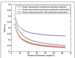
**Fig. 2** MSE performance comparison of estimating the target scattering matrix  $\mathbf{S}_{\rm t}$  versus the number of observation samples, with SCNR = 0 dB
