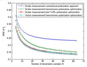
**Fig. 4** MSE performance comparison between scalar measurement systems and vector measurement ones versus the number of observation samples, with SCNR = 0 dB
