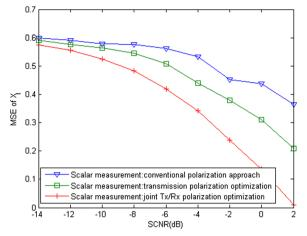
**Fig. 3** MSE performance comparison of estimating the target scattering matrix  $S_t$  versus the SCNR, with a fixed 50 observation samples
