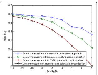
**Fig. 5** MSE performance comparison between scalar measurement systems and vector measurement ones versus the SCNR, with a fixed 50 observation samples
