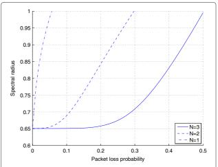
**Fig. 4** Spectral radius. Spectral radius  $\sigma_r(\mathfrak{A})$  of  $\mathfrak{A}$  in (34) for N=1,2,3 and as a function of the packet loss probability  $p \in [0,0.5]$
