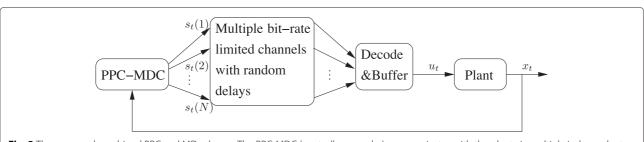
Fig. 2 The proposed combined PPC and MD scheme. The PPC-MDC (controller-encoder) communicates with the plant via multiple independent data-rate limited (digital) erasure channels with delays. The received descriptions are decoded and combined in the buffer
