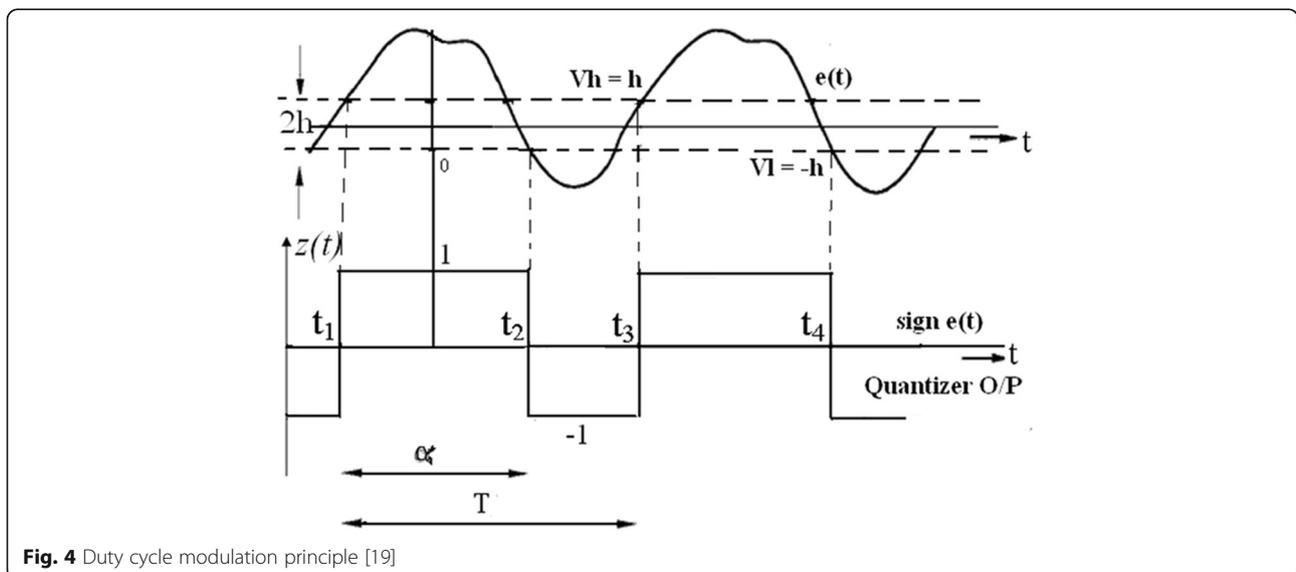
**Fig. 4** Duty cycle modulation principle [19]
