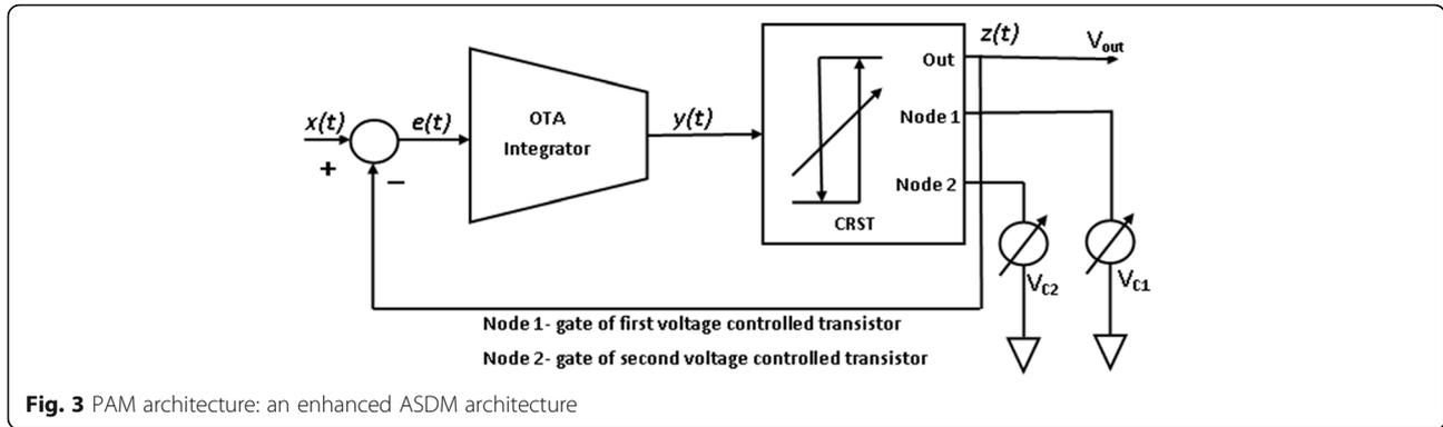
**Fig. 3** PAM architecture: an enhanced ASDM architecture
