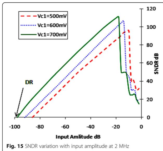
**Fig. 15** SNDR variation with input amplitude at 2 MHz
