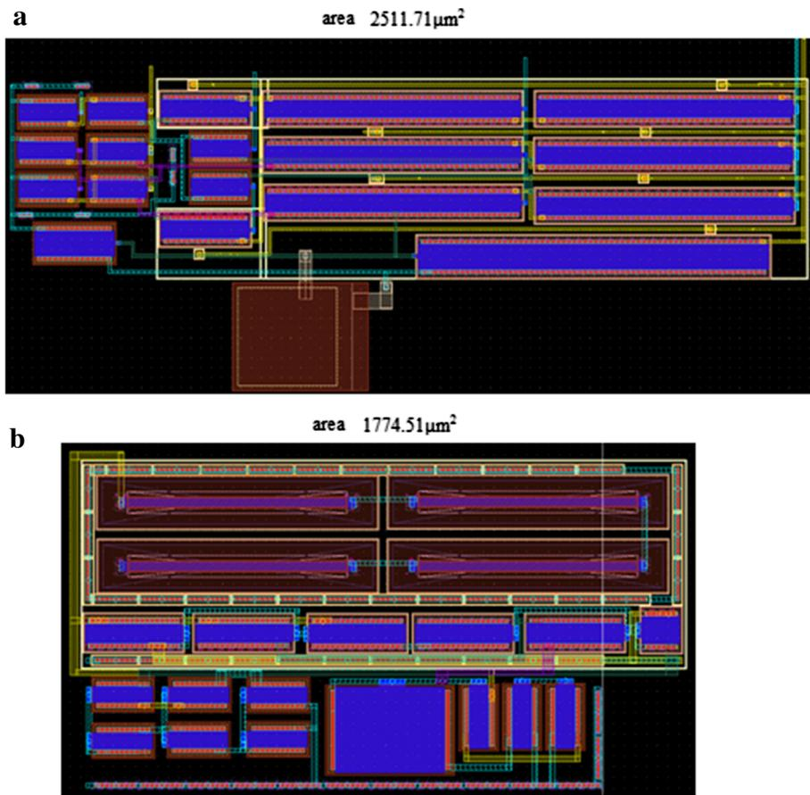
**Fig. 8** Layout design: (a) OTA, (b) bias circuit
