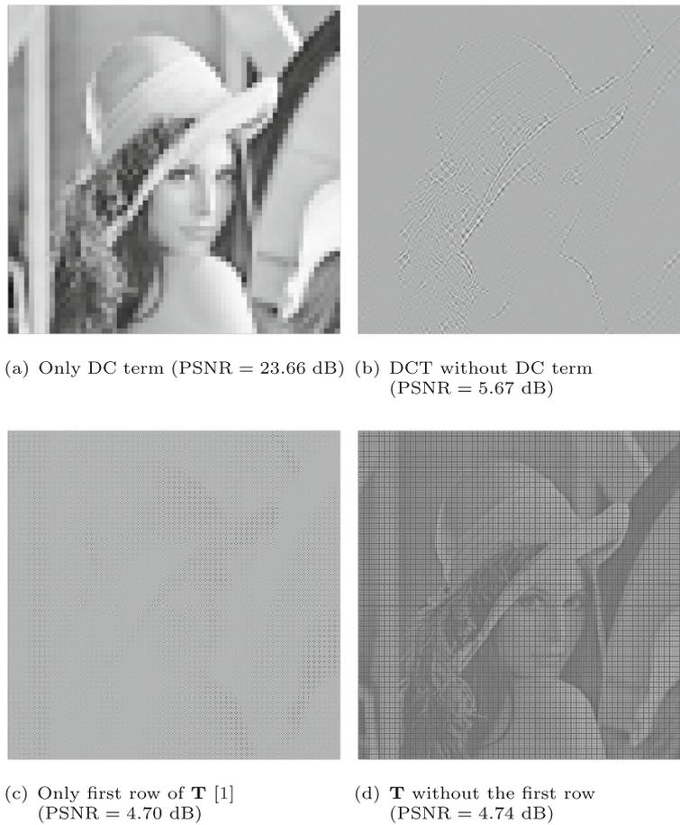
**Fig. 1** Reconstructed Lena image based **a** only on the DC component of the DCT, **b** on all DCT transform coefficient except the DC component, **c** only on the first row of the  $\mathbf{T}$  [1], and **d** on all  $\mathbf{T}$  coefficients, except the first row
