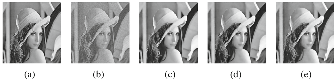
Fig. 13 Denoised results on Lena a original image; b Lena image corrupted with Gaussian noise with \sigma = 20 ; c restored image by optimal value of c = 1.69 ; d restored image by c = 1.78 ; e restored image by c = 1.61
