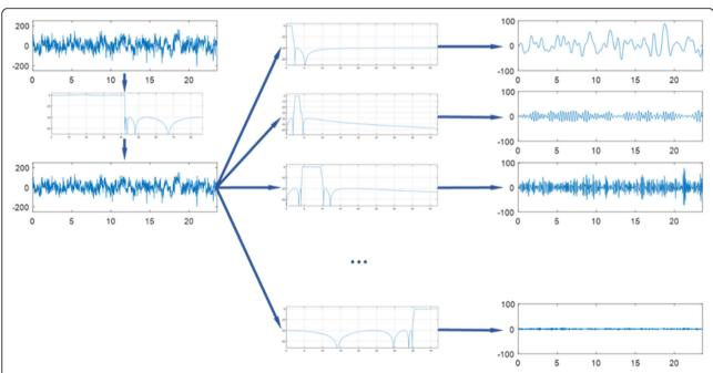
**Fig. 4** Spectral feature extraction step. After initial filtering (0–42 Hz), the signal is filtered with N+1 elliptic filters (middle column), resulting to N+1 filtered signals (right column)
