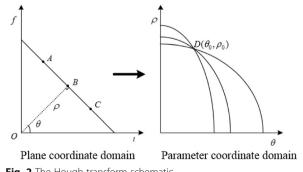
Fig. 2 The Hough transform schematic
