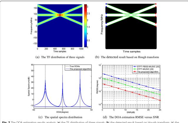
Fig. 7 The DOA estimation results analysis, (a) the TF distribution of three signals, (b) the detected result based on Hough transform, (c) the spatial spectra distribution, (d) the RMSE of DOA estimation versus SNR
