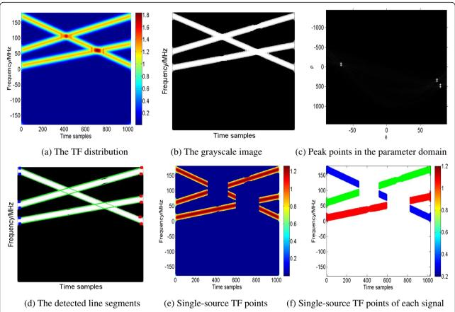
**Fig. 3** The single-source TF points selection method, (**a**) the TF distribution, (**b**) the grayscale image, (**c**) peak points in the parameter domain, (**d**) the detected line segments, (**e**) single-source TF points, (**f**) single-source TF points of each signal
