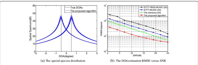
Fig. 5 The angular resolution of the proposed algorithm (DOA spacing: 1 °), (a) the spatial spectrum distribution, (b) the RMSE of DOA estimation versus SNR
