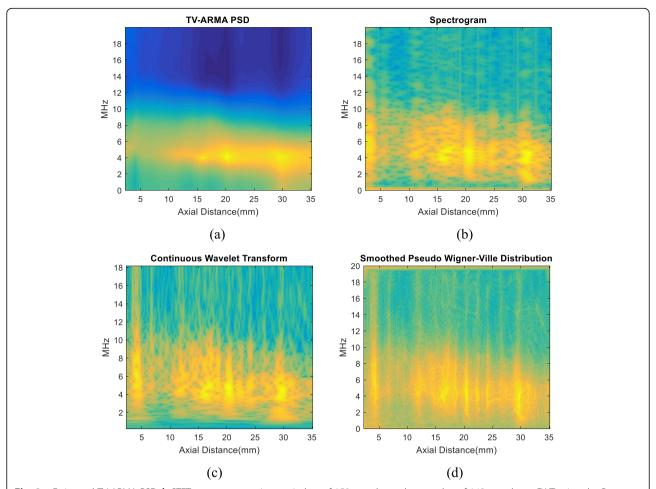
Fig. 9 a Estimated TV-ARMA PSD. b STFT spectrogram using a window of 150 samples and an overlap of 149 samples. c CWT using the Bump wavelet. d Smoothed pseudo-WVD
