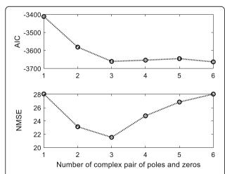
**Fig. 8** AIC score and NMSE between original and predicted (a posteriori) time series for an increasing number of complex pair of poles and zeros. The smallest AIC and NMSE value was achieved for three complex poles and three complex zeros
