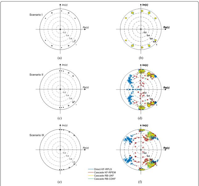
Fig. 4 Pole-zero plots of the actual simulated (left panel a, c, e) and estimated ARMA processes (right panel) for Scenarios I (upper panel), II (middle panel), and III (bottom panel). Blue, red, yellow, and green markers refer to direct-form models estimated by KF-RPLS and cascade-form models estimated by KF-RPEM, RB-UKF, and RB-CDKF, respectively
