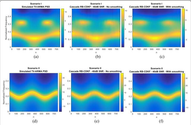
**Fig. 6** Simulated (**a**, **d**) and estimated (**b**, **c**, **e**, **f**) TV PSDs (averaged over all 30 realizations) for Scenario I (upper panel) and Scenario II (bottom panel), under 40 dB SNR and either with (right panel) or without (middle panel) smoothing. The estimation technique used was RB-CDKF combined with the cascade-form ARMA models
