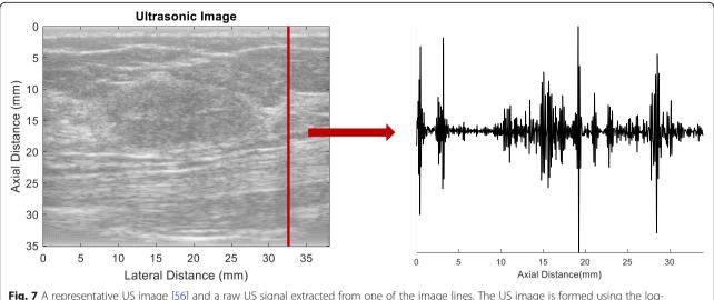
Fig. 7 A representative US image [56] and a raw US signal extracted from one of the image lines. The US image is formed using the log-compressed envelope of the raw US signals of each line
