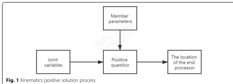
**Fig. 1** Kinematics positive solution process
