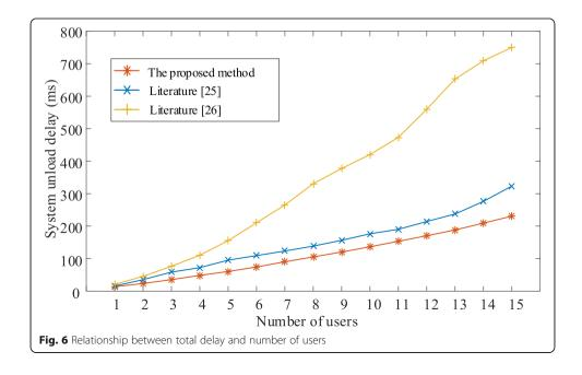
in literature [25] and literature [26] need to perform task offload sequence, and wait for other users to complete tasks before offloading. The offloading strategy method proposed in this paper can satisfy more users to offload tasks at the same time under limited channel resources.
