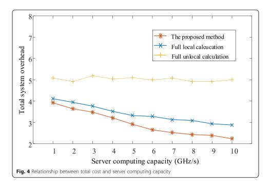
servers. Obviously, this is because the number of computing resources of MEC servers has no effect on the local computing process. The other two curves show a downward trend as F increases. This is because the larger F is, the server can allocate more computing resources to users, thereby reducing processing time and energy consumption. The curve of DQN method proposed in this paper is always at the bottom and performs best.
