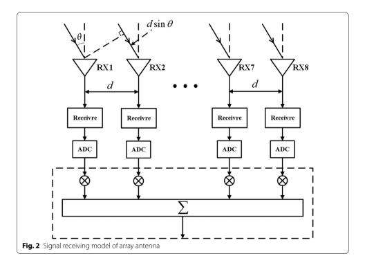
Based on the above equation, the phase change of the *i*-th receiving antenna is
