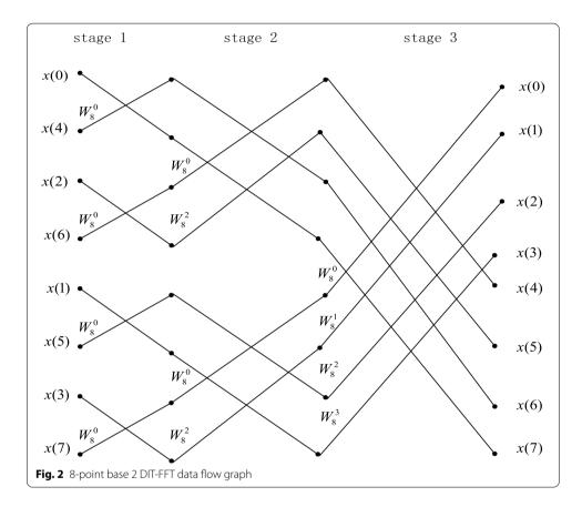
decomposed. Where N is an integer power of 2. The corresponding 8-point base 2 DIT-FFT iteration process is shown in Fig. 1. The 8-point base 2 DIT-FFT data flow diagram is shown in Fig. 2, which has 3 stages and a total of 16 butterfly cells. Note that the input and output are a bit reversed, with the input in reverse order and the output in positive order.
