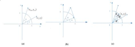
**Fig. 3** Rotation mode of CORDIC algorithm in a circular system. **a** Vector rotation; **b** vector pseudo rotation; **c** it breaks down into smaller angles
