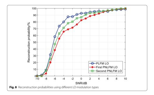
sampling schemes are the same as those in Fig. 5. The signals in group 3 in (44) are the intercepted signals. Figure 8 demonstrates the reconstruction probability using different LO modulation types.
