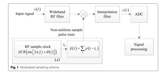
pass band is  $f_s$ . At last, the filtered signal y(t) is sampled again by an ADC with a low sample rate that satisfies the Nyquist sampling theorem.
