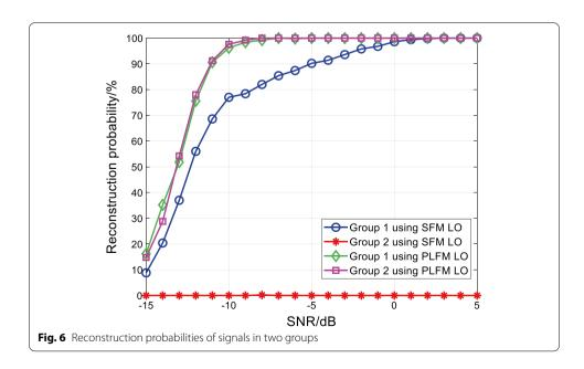
Figure 6 demonstrates the reconstruction probabilities of the two groups using the two LO modulation types.
